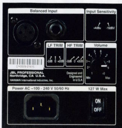
The rear-panel controls for bass and treble response, level and input sensitivity are common to both the LSR305 and LSR308.
